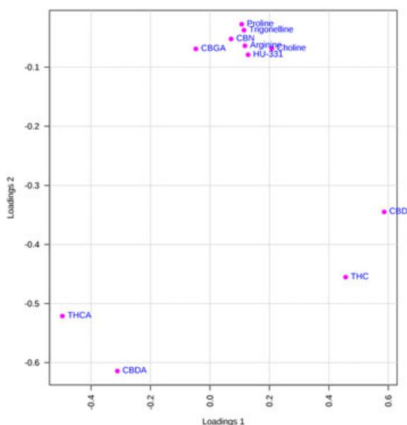
**Figure 4.** Principal component analysis (PCA) loadings of identified metabolites in ethyl alcohol cannabis medicinal extracts (CMEs) in ESI+ mode. Compounds with loadings far from zero (positive or negative) have a stronger contribution to creating the clusters separation. [Colour figure can be viewed at [wileyonlinelibrary.com](http://wileyonlinelibrary.com)]
