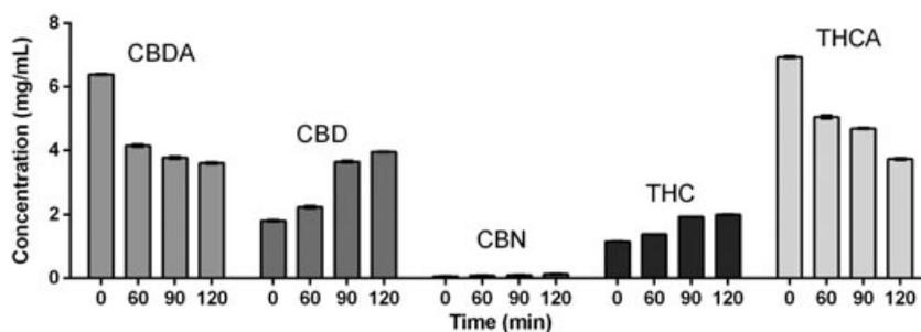
**Figure 8.** Cannabinoids concentration in ethyl alcohol at the different extraction time points. Cannabinoids concentrations (mg/mL, y axis) in ethyl alcohol acquired in ESI+ mode were plotted against time of extraction (min, x axis).
