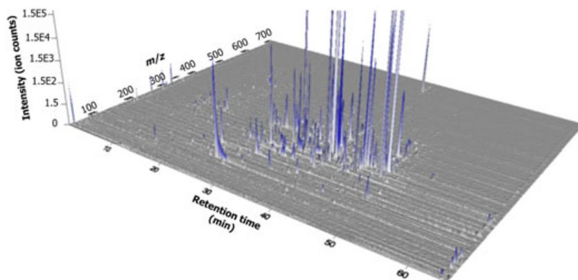
**Figure 1.** Three-dimensional (3D) total ion chromatogram (TIC) of an alcohol cannabis medicinal extract (CME) at 60 min in negative ionisation (ESI-) mode. The retention time (min) is represented on the x axis, the peak intensity (ion counts) on the y axis and the *m/z* values on the z axis. [Colour figure can be viewed at [wileyonlinelibrary.com](http://wileyonlinelibrary.com)]
